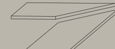
ANGOLARE ESTERNO BORDO TORO EXT. BULLNOSE EDGE CORNER / ANG. EXT. CHANT ARRONDI / AUSSENECKTRITTSTUFE / ANG. EXT. CANTO ROMO ▲ 60x120 (24"x48") RT 20mm ▲ 30x120 (12"x48") RT 20mm ▲ 30x60 (12"x24") RT 20mm
